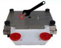
Remove the screw under the balance
