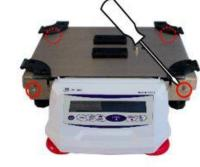
Remove the screws placed on the corners (n°4)
