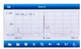
Spectrum scan and detection of peaks
